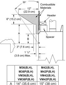
Figure 5 - Mantel Clearances - Side View (Cross Section)
